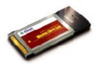
Complying with the 802.11g standard, the WL-3565 provides a faster wireless connection for laptop users who access network resources. Moreover, the WL-3565 supports specific ways to increase the data transfer rate at a time, compressing the data and decreasing the waiting time to send the next data to the Routers or APs. This feature is called Turbo Mode. When the card is connecting to the Routers or APs with the proprietary Turbo Mode feature, the wireless network will be more effective.
